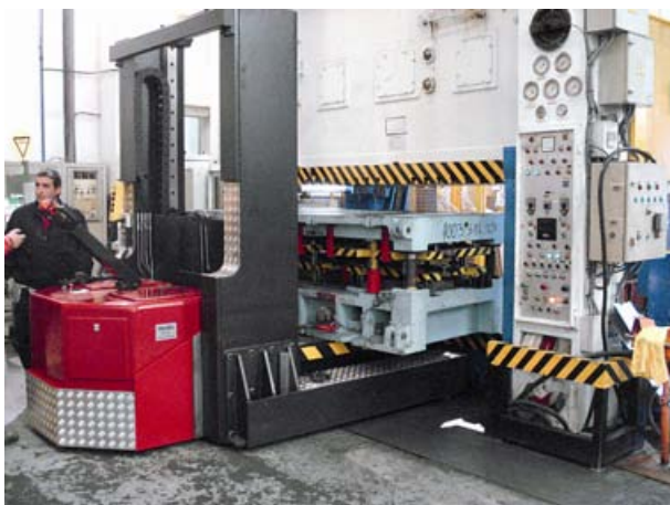
A Die Change Cart type "Front Loader" with high lift during change of press die at a press with a very low press table. In this case the high lift is needed for the die rack.
