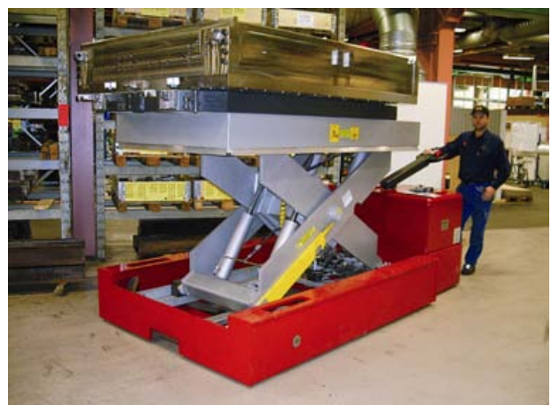
A Die Change Cart type "Front Loader" with high lift, execution by scissor lift
