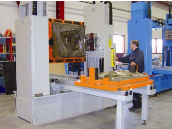
Splitting of a press die within a small Die Splitter with 2-column-design. The upper part of the die is rotated by 90°.
