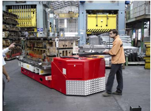
Training of an operator how to use the Die Change Cart
