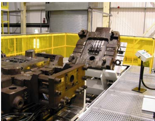
Heavy size Plastic Injection Mould Splitter during turning of the 2nd half of a 40 tons mould after opening
