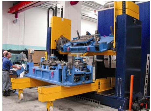
Turning of an upper part of a press die within a middle size Die Splitter, whilst the lower part of the press die is lying on the floor beams of the splitter, accessible for the operator
