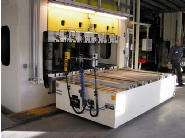
Rail based battery driven Die Change Cart for heavy press dies
