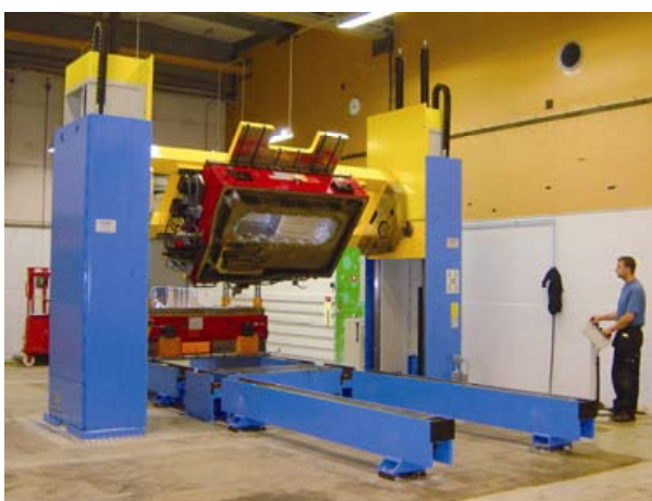
Middle size Die Splitter for press dies up to 30 tons weight
