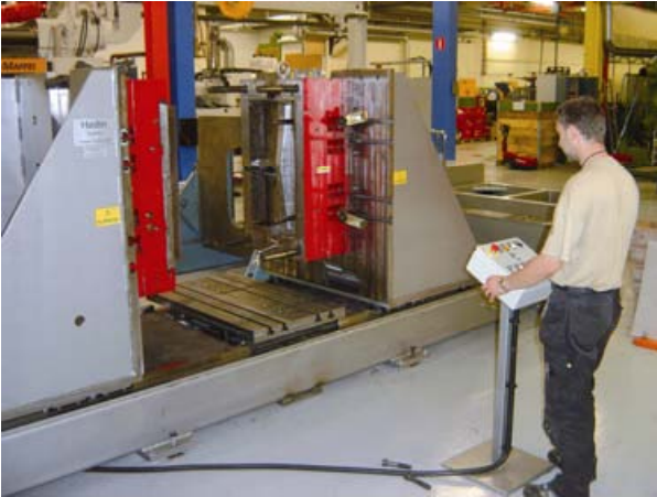
Light size Mould Splitter for opening and splitting of moulds.
