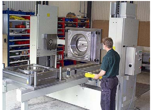
Light Die Splitter with feeding of the press die via die loading arms, equipped with pneumatic die lifters with rollers. Also movable die loading arms to suit wide dies.
