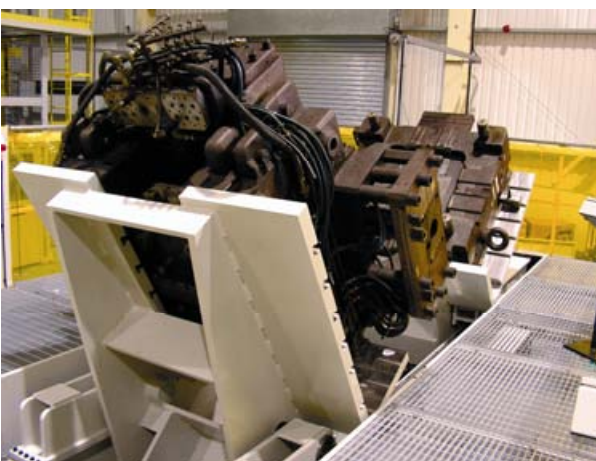
Heavy size Mould Splitter for opening of the mould and turning of each of the halves of the mould by 90°
