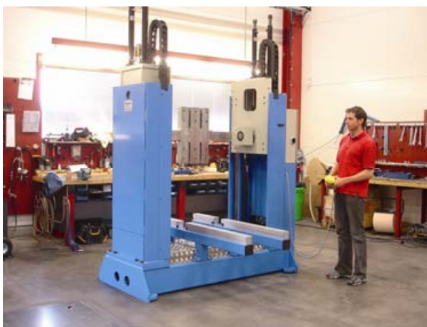
Light Die Splitter up to 3 tons load capacity as a 2-column-design
