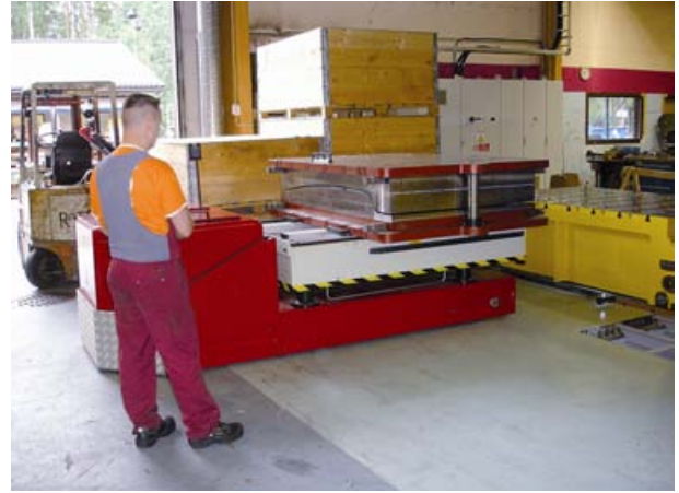
Testing of a Die Change Cart type "Front Loader" with low stroke before delivery
