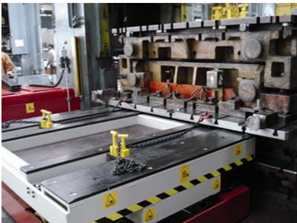
A Die Change Cart type "Side Loader" with low stroke during pulling a press die out of the press
