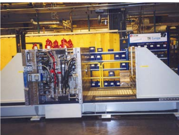
Opening stroke of a middle size Plastic Injection Mould Splitter without turning function
