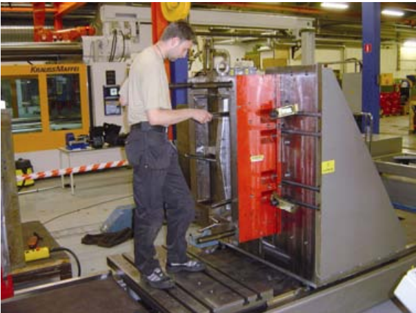
Maintenance work on an opened mould on a small Plastic Injection Mould Splitter
