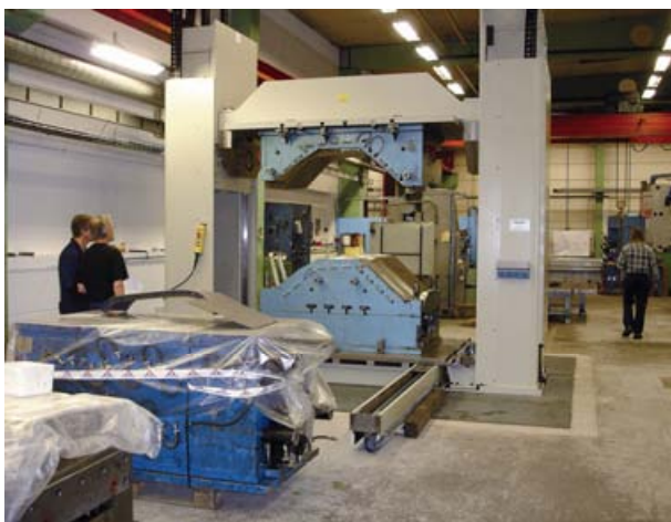
Use of a Hedin Die Splitter within the production process of an RTM production line, with heavy moulds for glassfiber products
